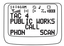
This figure is typical of what you see on your radio. The 64 x 96 pixel liquid crystal display (LCD) shows radio status, text, and menu entries.
