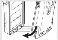
Press both sides at the top of the battery against the radio until both latches click into place.
