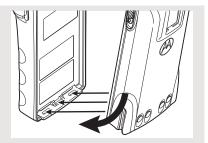
2 Press the top of the battery against the radio until both latches click into place.
