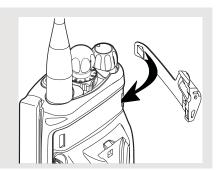
2 Snap the larger end of the adapter into place in the shroud indent, below the antenna port.
