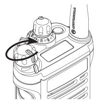
If the power-up test is successful, you see momentary **SELFTEST** on the radio's display, followed by the Home screen. Turn off the radio, check the battery, and turn the radio back on. If the radio fails the power-up test again, record the **Error XX/YY** code and contact your dealer.
