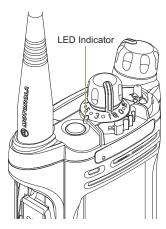
The LED lights up solid red while the radio is transmitting. In conventional mode, the LED lights up solid yellow when the radio is receiving a transmission. In trunking mode, there is no LED indication when the radio receives a transmission.
