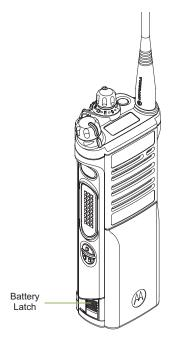
To remove the battery, turn the radio off. Squeeze the release latches at the bottom of the battery until the battery releases from the radio. Remove the battery from the radio.
