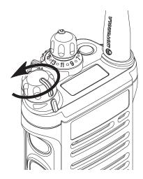
To turn off the radio, rotate the **On/Off/Volume Control Knob** counterclockwise until you hear a click.
