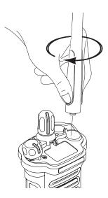
To remove the antenna, turn the antenna counterclockwise. Make sure you turn off the radio first.
