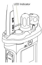
The LED lights up solid red while the radio is transmitting. In conventional mode, the LED lights up solid yellow when the radio is receiving a transmission. In trunking mode, there is no LED indication when the radio receives a transmission.
