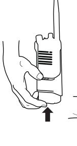
To remove the radio from the carry holder, place the tip of your fingers on the ledge of the carry holder and push at the bottom of the radio until the radio is released from it.
