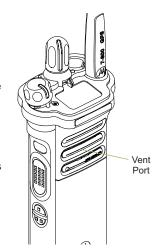
The APX 6000XE radio is designed to be submerged to a maximum depth of 6 feet, with a maximum submersion time of 2 hours.
