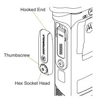
Rotate and lift the connector cover to disengage it from the radio.
