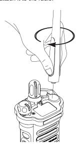
To remove the antenna, turn the antenna counterclockwise. Make sure you turn off the radio first.
