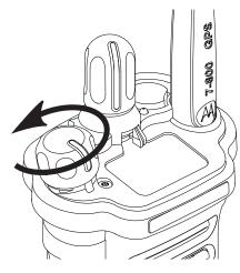
To turn off the radio, rotate the **On/Off/Volume Control Knob** counterclockwise until you hear a click.
