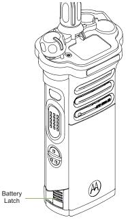
To remove the battery, turn the radio off. Squeeze the release latches at the bottom of the battery until the battery releases from the radio. Remove the battery from the radio.
