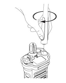
To remove the antenna, turn the antenna counterclockwise. Make sure you turn off the radio first.
