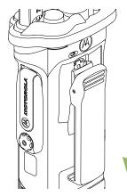
To remove the clip, use a flat-bladed object to press the belt clip tab away from the radio. Then, slide the clip downward and away from the radio.
