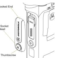
To remove the accessory connector cover, rotate the thumbscrew counterclockwise until it disengages from the radio. If the thumbscrew is too tight, use an Allen wrench to loosen it first.
