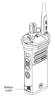
To remove the battery, turn the radio off. Squeeze the release latches on the bottom of the battery until the battery releases from the radio. Remove the battery from the radio.
