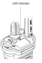
The LED lights up solid red while the radio is transmitting. In conventional mode, the LED lights up solid yellow when the radio is receiving a transmission. In trunking mode, there is no LED indication when the radio receives a transmission.
