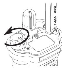
To turn off the radio, rotate the **On/Off/Volume Control Knob** counterclockwise until you hear a click.
