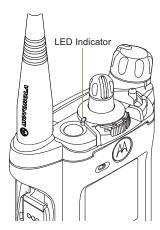
The LED lights up solid red while the radio is transmitting. In conventional mode, the LED lights up solid yellow when the radio is receiving a transmission. In trunking mode, there is no LED indication when the radio receives a transmission.
