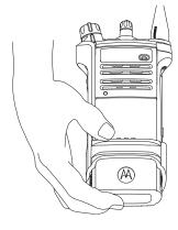
To remove the radio from the carry holder, place the tip of your fingers on the ledge of the carry holder and push at the bottom of the radio until the radio is released from it.
