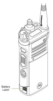
To remove the battery, turn the radio off. Squeeze the release latches at the bottom of the battery until the battery releases from the radio. Remove the battery from the radio.
