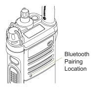
The range of Bluetooth operation is 10 meters line-of-sight communication. This is an **unobstructed** path between the location of the signal transmitter (your radio) and the location of the receiver (your device or accessory).
