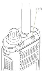
The LED lights up solid red while the radio is transmitting. In conventional mode, the LED lights up solid yellow when the radio is receiving a transmission. In trunking mode, there is no LED indication when the radio receives a transmission.
