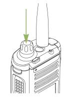
To turn off your radio, press and hold the MFK until the radio display shows **Power off?**, press the **Menu Select** button below **Yes** to power off.
