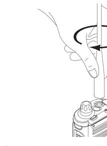
To remove the antenna, turn the antenna counterclockwise. Make sure you turn off the radio first.
